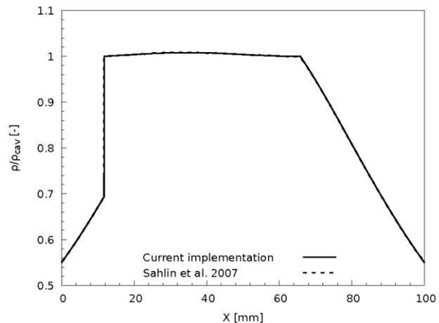
Fig. 6 Fluid density ratio for  $\rho_w/\rho_{cav} = 0.55$  in case of the single parabolic slider.
