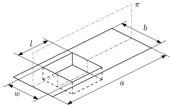
**Fig. 10** Microtexture pocket bearing geometry [11].
