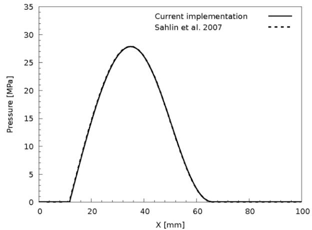
Fig. 7 Fluid pressure for  $\rho_w/\rho_{cav} = 0.55$  in case of the single parabolic slider.
